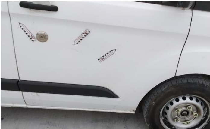
11: Door nsr Dented With Paint Damage
