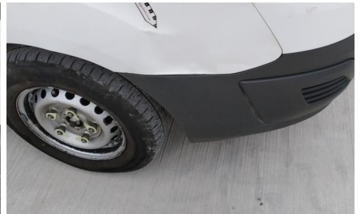
12: Qtr Panel osr Dented With Paint Damage
