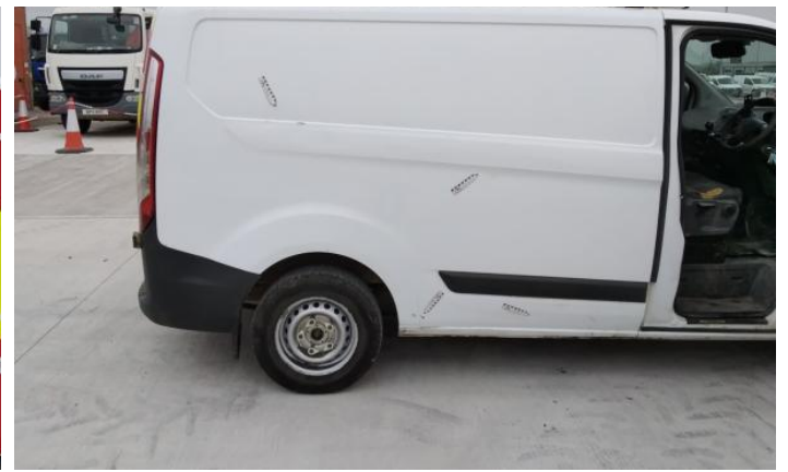
10: Qtr Panel osr Scratched Over 25mm Thru Paint
