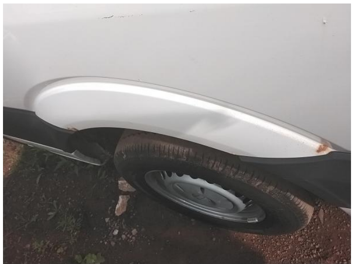
20: Qtr Panel osr Dented Over 30mm
