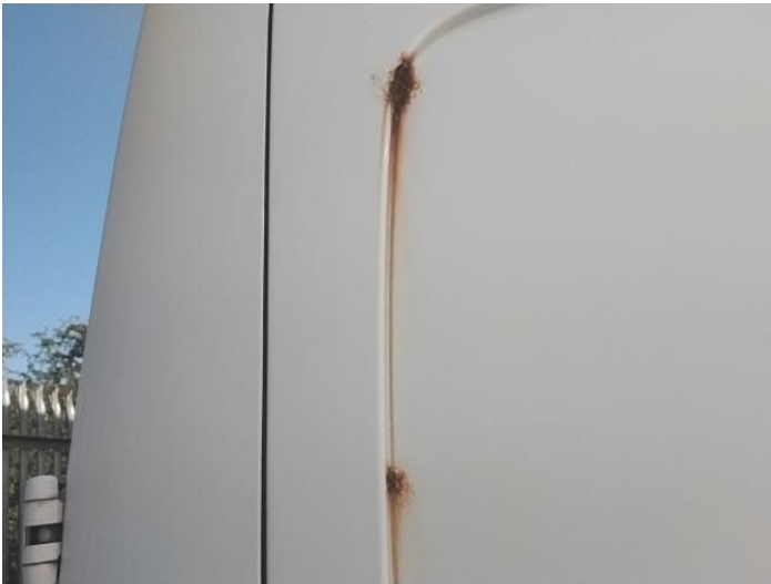
17: Qtr Panel osr Rusted Over 5mm
