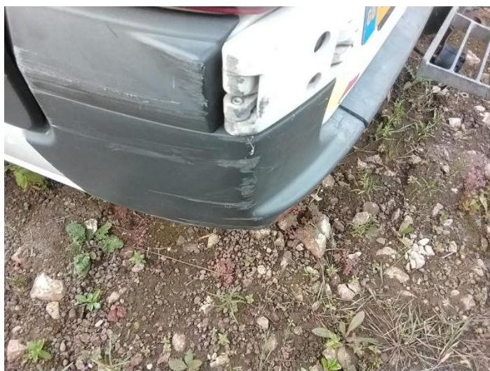
14: Bumper Rear Moulding Scuffed (Unpainted) Over 100mm
